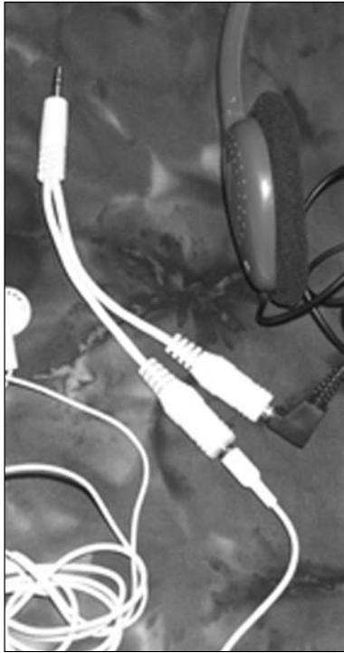
Figure 2-5: A head- phone cable that splits into two, allowing two sets of headphones.
